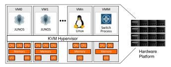
Figure 3:- Basic Cloud Structure
